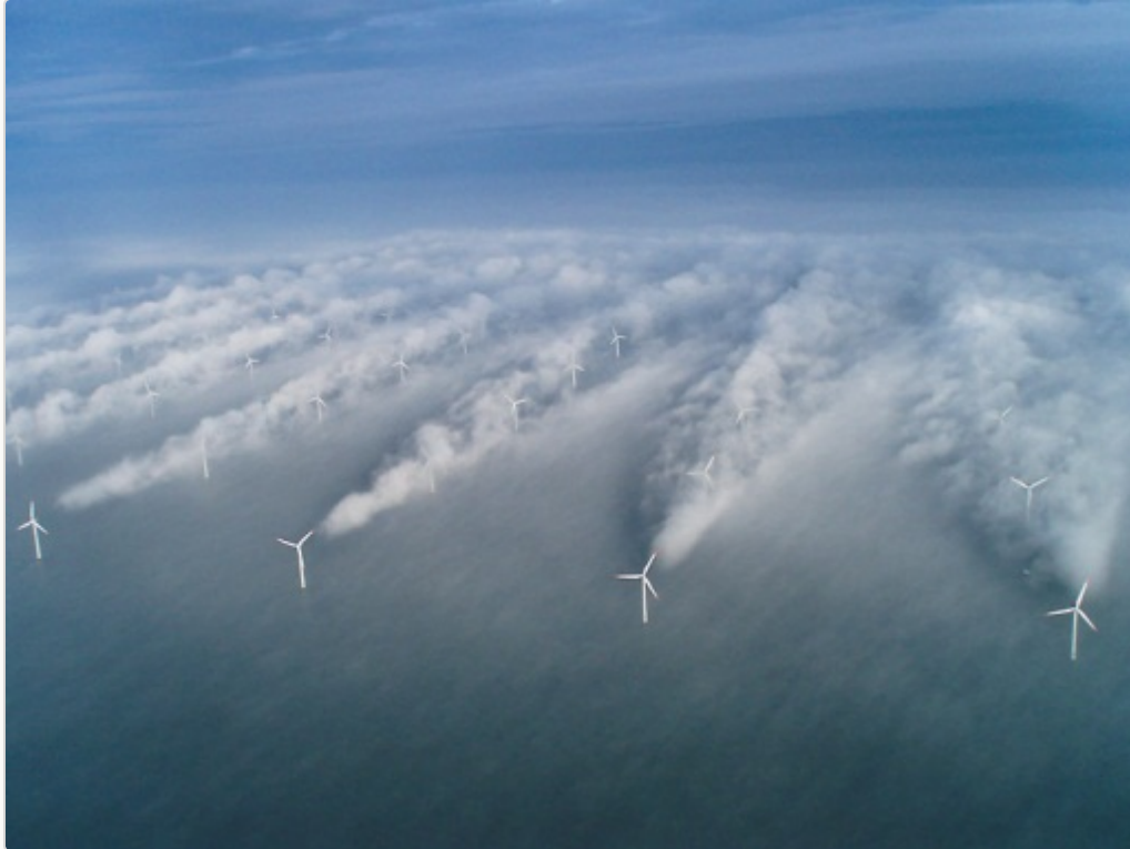
Visible wakes behind offshore turbines. Photograph reproduced from original PowerPoint, slide 43, which credits WindAction.
